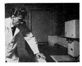
OPERATOR Ron Cheek watches the light head project beam of light on film (white dot under the light head at right). The beam is computer controlled to "draw" the circuit on film.
